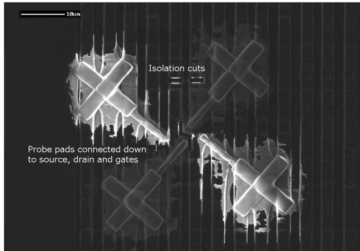
Image - Floating and grounded probe pads connected to gates, source and drain of a transistor pair.
