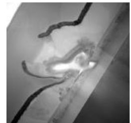
TEM SE image of a FIB prepared TEM section through the same embedded insulative defect.
