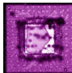
Acoustic microscopy scan of a BGA packaged part with die attach delamination visible.
