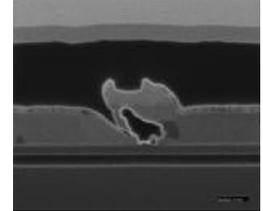
Ion beam secondary electron image of a FIB microsection through an embedded insulative defect.
