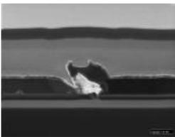
**SIM SI** (w/secondary ion imaging) - all the benefits of SIM SE imaging but with less sample charge sensitivity, more materials information and no voltage contrast. Great for understanding insulative defects and can be used with charge neutralisation on fully insulative samples.
