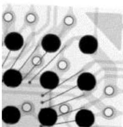
**X-ray imaging** - normal or tilted, gives terrific non-destructive data about the internal structure of a device, its bonding, leads and connections. Very effective on board structures and solder connections.
