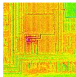
Delta R image of a voltage regulator using  $<0.5\mu\text{A}$  more current than expected (fail state).
