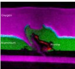
**200kV TEM EDS Mapping** gives high resolution elemental maps with a low interaction volume providing an optimised pixel size. The exact placement and custom orientation of our FIBxTEM sections produces the clearest picture of which-material-is-where at the smallest geometries. In this case from below the surface of the sample.
