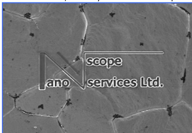
Image: a 12 µm wide 'NanoScope Services' logo ion beam milled onto a aluminium bond pad (showing metal grains, variable milling rates, boundary contamination and surface roughness)
